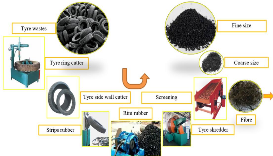
Fig (1): Preparation stages of the coarse and fine aggregates scrap tire wastes (A.M. Mhaya et al 2020)
